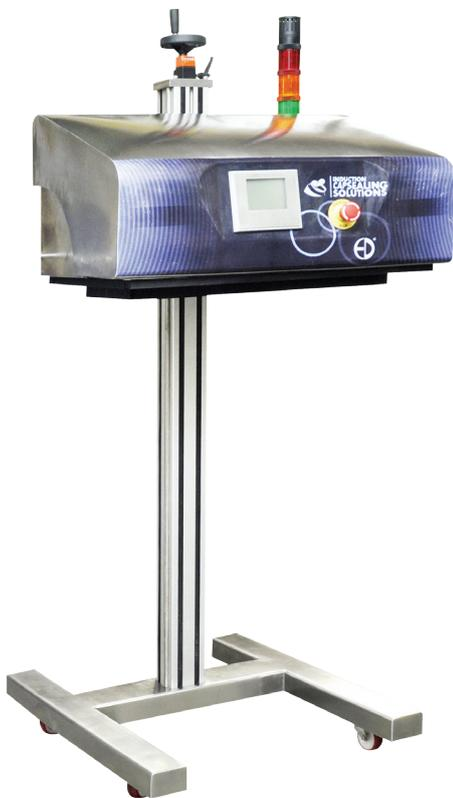
Touch Screen control for inspection & rejection.
